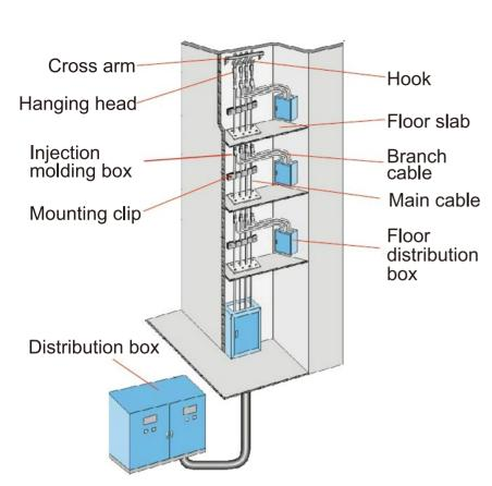
The passage of time and growing prosperity have led to more and higher buildings being built, resulting in greater electricity consumption. In the course of this development, it has also become increasingly difficult to wire buildings. The timely introduction of pre-branch cables has greatly reduced the installation time for trunk lines and the overall cost of construction projects.
